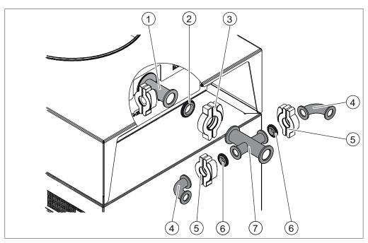
Fig. 11: Fitting the cross-pipe
