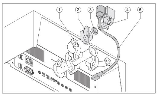
Fig. 16: Fitting the pressure-regulating valve
