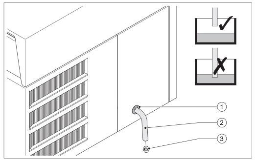
Fig. 18: Condensate drain hose
