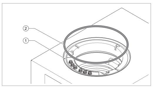
Fig. 20: Fitting the 300 mm dia. O-ring
