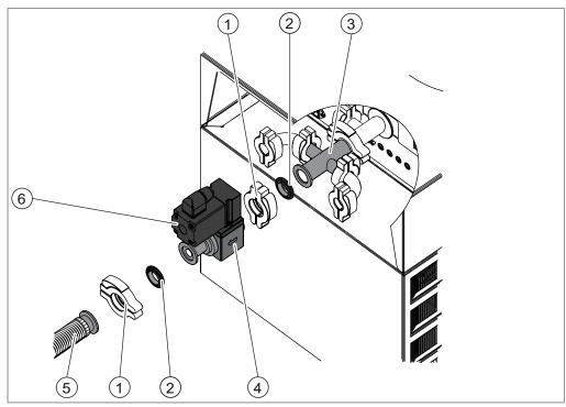
Fig. 12: Fitting the main valve
