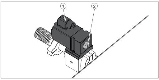
Fig. 13: Manual switch on main valve
