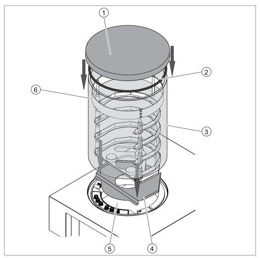
Fig. 21: Fitting the acrylic drying chamber
