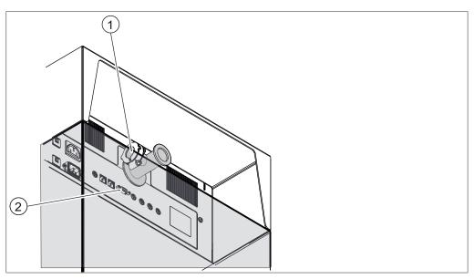
Fig. 17: Fitting alternative pressure sensor
