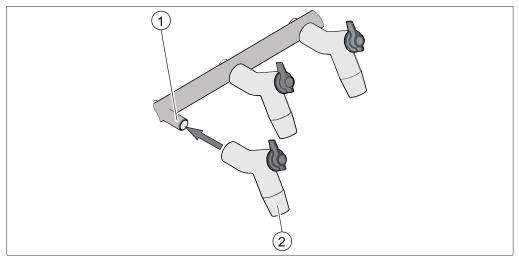
Fig. 32: Fitting manifold valves
