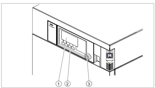
Fig. 5: Basic control panel
