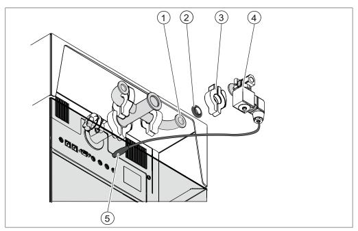
Fig. 15: Fitting the venting valve
