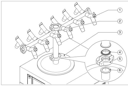
Fig. 24: Manifold drying rack
