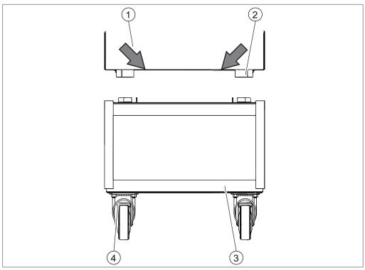
Fig. 9: Lifting the instrument
