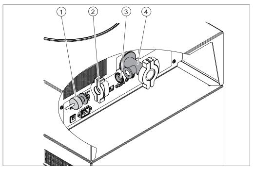
Fig. 14: Fitting the pressure sensor
