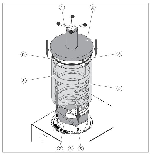
Fig. 23: Fitting the stopper acrylic drying chamber
