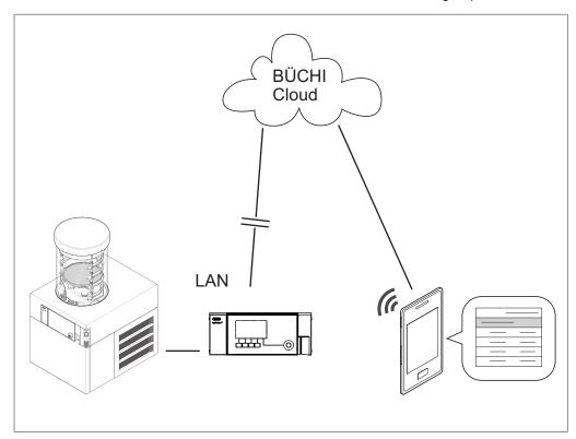
The BUCHI Connect Solution allows processes to be tracked and analysed from a mobile device while in progress.
