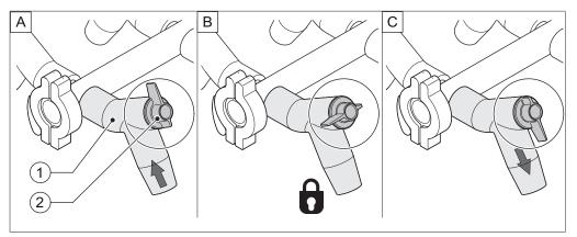
Fig. 33: Manifold valve
